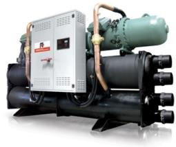
High efficiency unit for indoor installation for chilled water production. Semihermetic screw compressors optimized to operate with low compression ratio and R513A; shell and tubes condenser, flooded evaporator and electronic expansion valve. High efficiency unit thanks to the innovative optimized compressors and the high performing heat exchangers.
